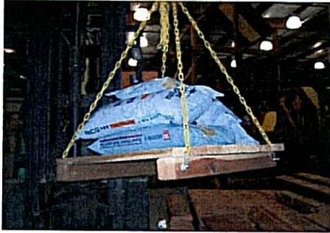
Conclusion: The purpose of this test was to gauge the structural integrity of our barrier. A pulley was used to change direction of force in a horizontal direction. The barrier tested was attached according to installation instructions. An inspection of the barrier was done prior to the test. There were no visible cracks or deformations before or after the test. A load of 136 pounds was applied laterally to the top rail, which surpasses the requirement of 125.4 pounds.
