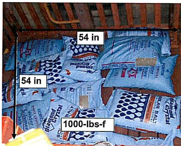
Conclusion: Structural integrity of the platform was tested using the calculation outlined in section B.3.2. A pre-test inspection was performed. The platform was assembled according to assembly instructions. A load of 1000 lbs was applied to the platform and left for 5 minutes. A post-test inspection was performed, and there were no visible deformations.
