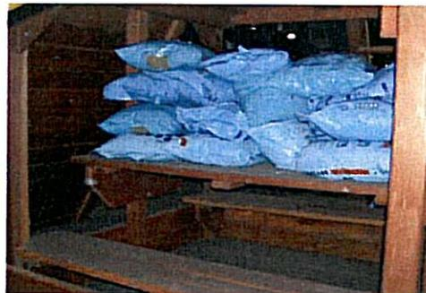
Conclusion: Structural integrity of the picnic table top platform was tested using the calculation outlined in section B.3.2. A pre-test inspection was performed. The platform was assembled according to assembly instructions. A load of 760 lbs was applied to the platform and left for 5 minutes. A post-test inspection was performed, and there were no visible deformations.
