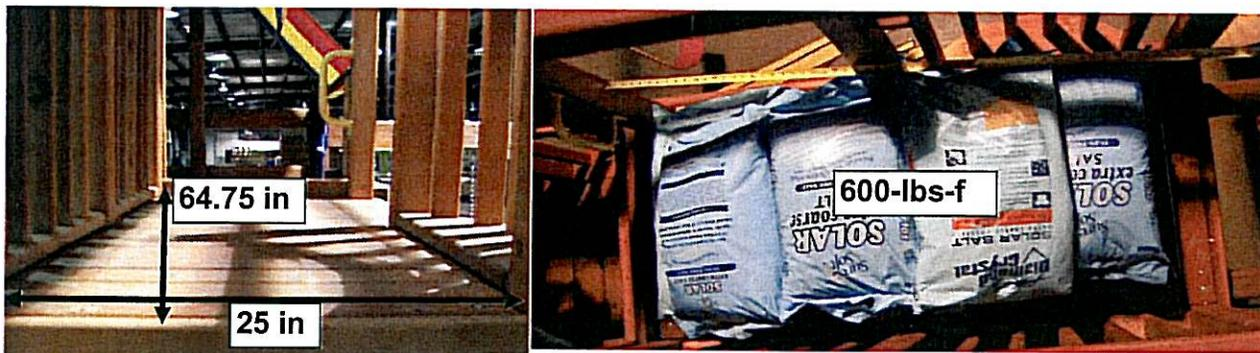
Conclusion: Structural integrity of the penthouse platform was tested using the calculation outlined in section B.3.2. A pre-test inspection was performed. The platform was assembled according to assembly instructions. A load of 600 lbs was applied to the platform and left for 5 minutes. A post-test inspection was performed, and there were no visible deformations.
